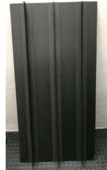
Composite demonstrator produced by AFP followed by LRI in one-shot
