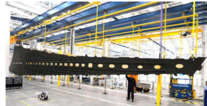
A350 XWB 32m by 6m lower wing cover
