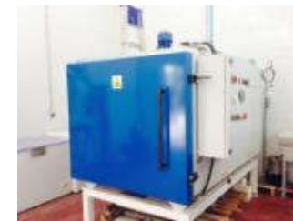
Composite curing oven for LRI process
