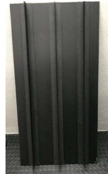
Composite demonstrator produced by AFP followed by LRI in one-shot
